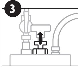
Lift seal on flask to draw up chemical under vacuum
