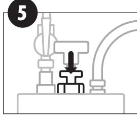
Release valve to break vacuum seal
