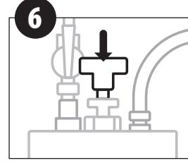
Depress spring on drain valve to release measured chemical
